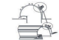
Step 03: Fix the frame on profile
