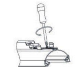
Step 01A: Fix the internal clips and the driver
