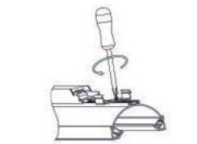
Step 03B: Fix the internal clips and the driver
